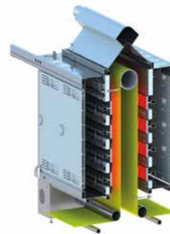
High-temperature oven for thermal treatment of carbon fabrics.
